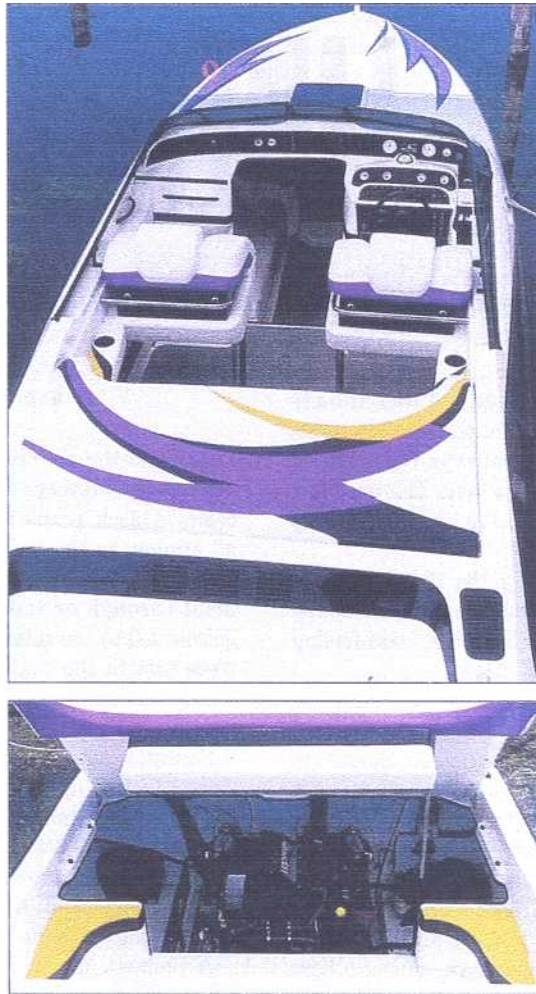
Space-galore—the engine compartment housed a Merc 502 Magnum protected by a power hatch and sunlounge.
